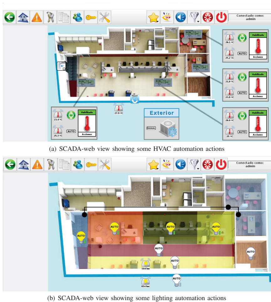
Figure 2. Rules implemented through the SCADA-web over the automated floor of the reference smart building
