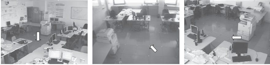
FIGURE 17.5 An example of point correspondence in the three different views employed for the offline camera calibration phase.
