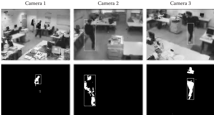
FIGURE 17.7 Local tracking results obtained by sensor agents ( t=200 s).
